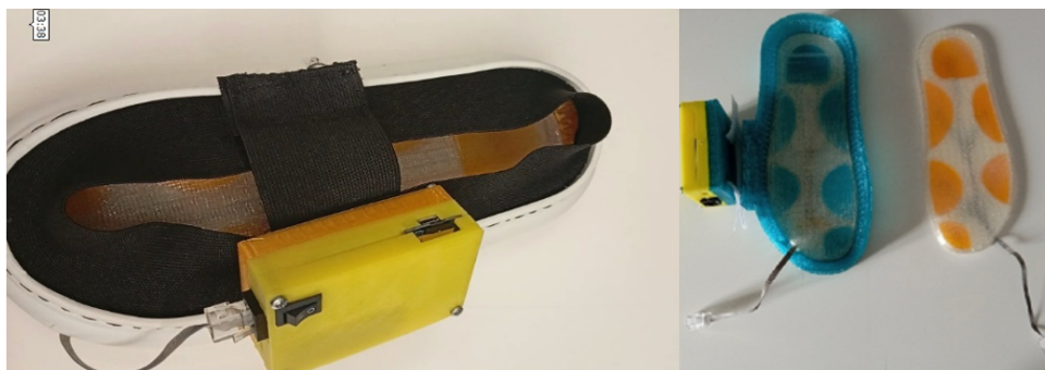
Figure 2: Developed flexible sensor-based shoe and electronic measurement hardware (EU size 36).
